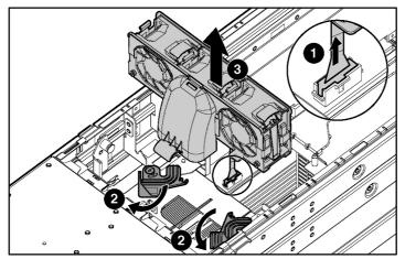
Figure 1-6: Removing the three-fan assembly
